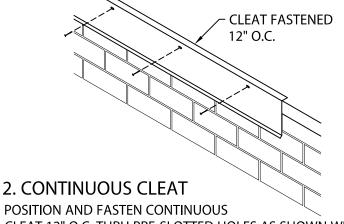
POSITION AND FASTEN CONTINUOUS CLEAT 12" O.C. THRU PRE-SLOTTED HOLES AS SHOWN WITH PROVIDED NAILS. LAP CLEAT 1" AT JOINTS.
