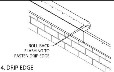
**ROLL BACK FLASHING TO EXPOSE FASTENING SLOTS** AND FASTEN THRU PRE-SLOTTED HOLES 6" WITH PROVIDED NAILS.
